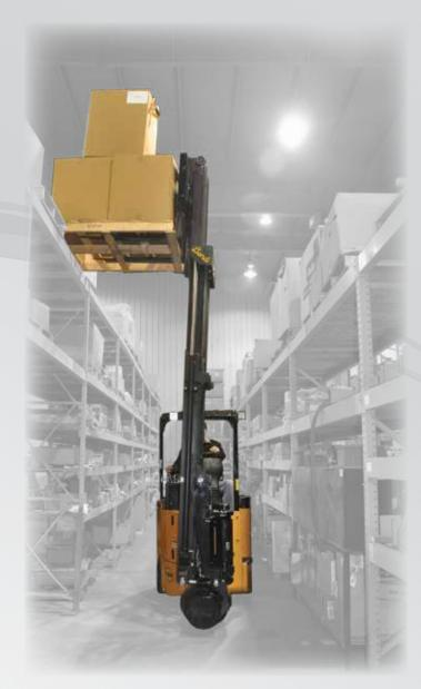
The B3/30 is a 3-wheel Bendi, with a single poly front drive tire and solid rubber rear tires. Front articulation of 200°, narrow mast and compact front end allows stacking easily in Very Narrow Aisles. The B3/30 can also work inside and outside on paved surfaces.
