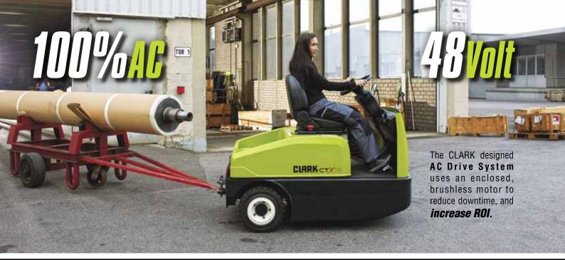
The **100% AC** 48-Volt high performance drive system, and regenerative braking, give the compact rear-wheel drive CTX exceptional *acceleration, speed,* and *gradeability*.
