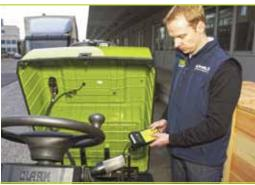
• The CLARK handset can be used for diagnostics and settings of up to 20 different performance parameters to match your requirements.
