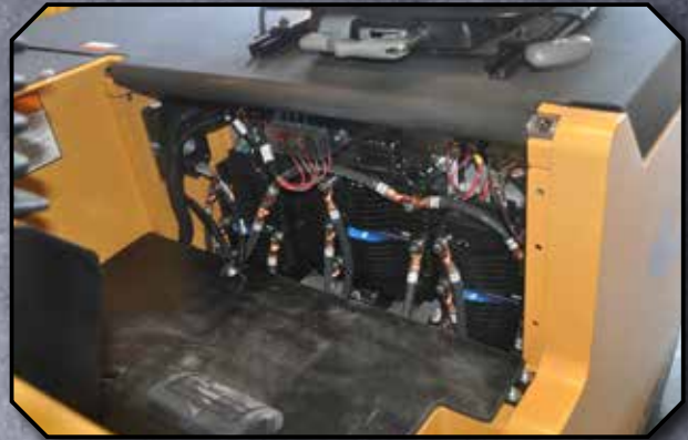
Removeable Cover Provides Easy Access to All Control Components
