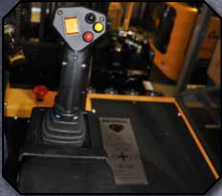
Single Joystick Controls for All Hydraulic Functions, Directional Control and Horn
